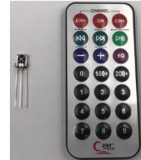
Fig. 6. Infrared reception and infrared remote control
